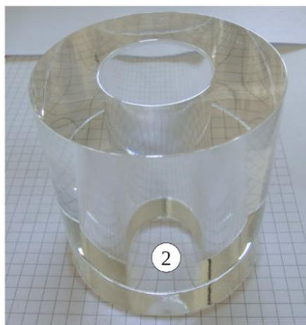
Quartz cylinder (thick-walled) for pressures up to 50 bar
