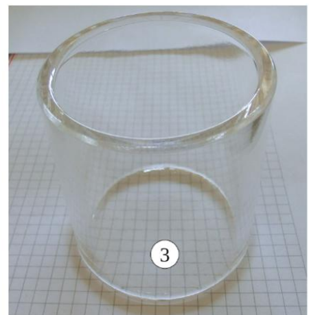
Quartz cylinder (thin-walled) for pressures up to 10 bar
