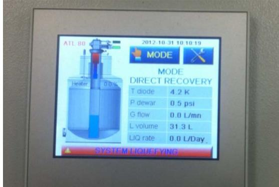
**Figure 4 (left) Liquid helium transfer from ATL80 to PPMS system (right) Control screen showing liquefaction**
