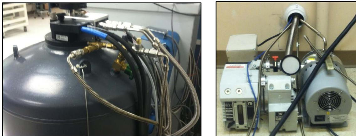
**Figure 3 PPMS recovery lines: (left) Bath boil off (right) Output from annulus via scroll pump**
