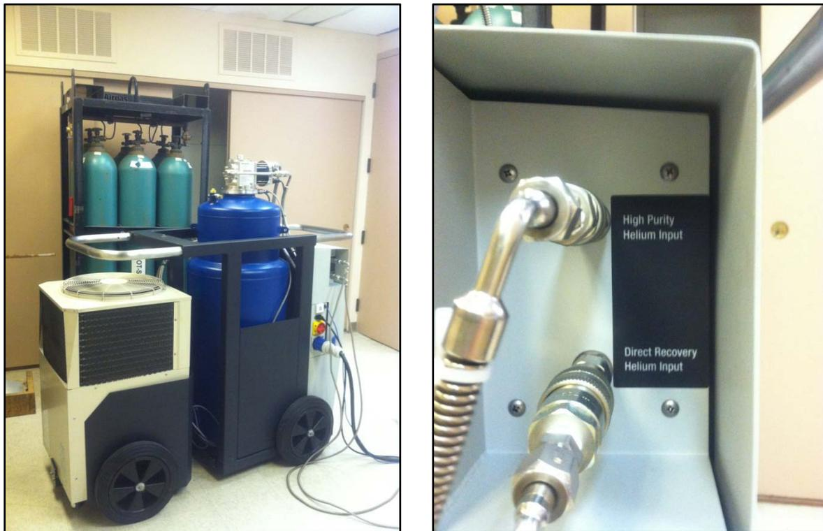
**Figure 2 (left) ATL80 connected with PPMS and 6-pack of helium cylinders (right) Dual gas inputs on ATL80**
